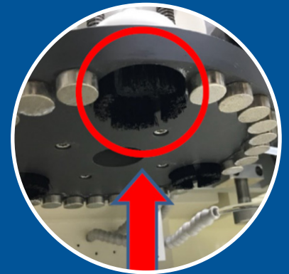
Nylon Brush with High Pressure Spray Nozzle for pad cleaning
