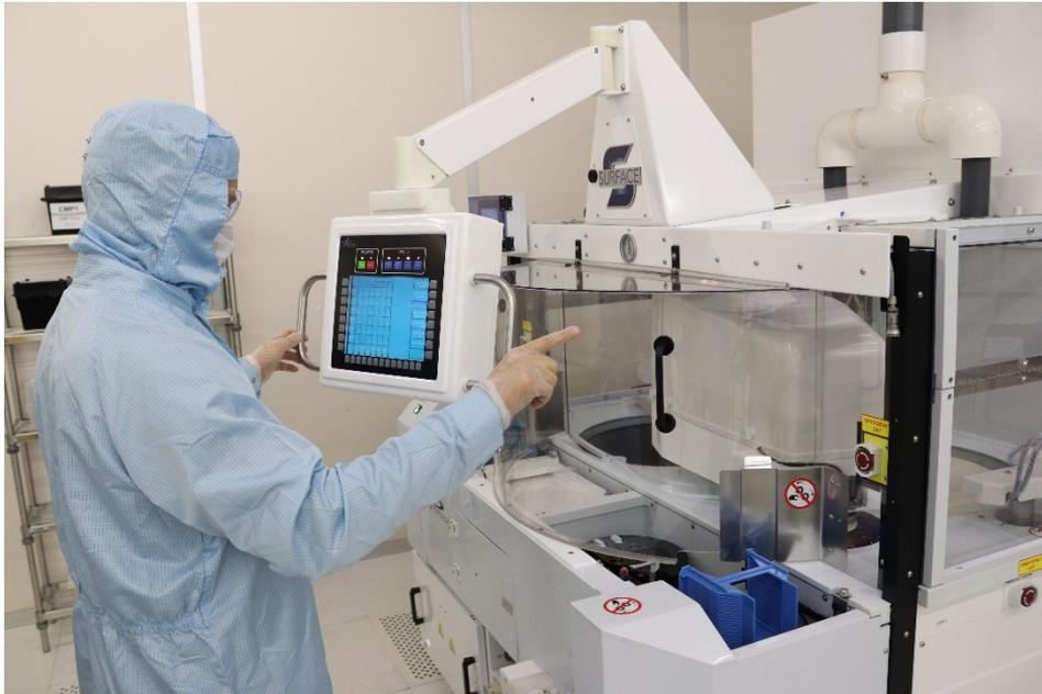
*Chemical Mechanical Polishing tool from Axis Technology*
