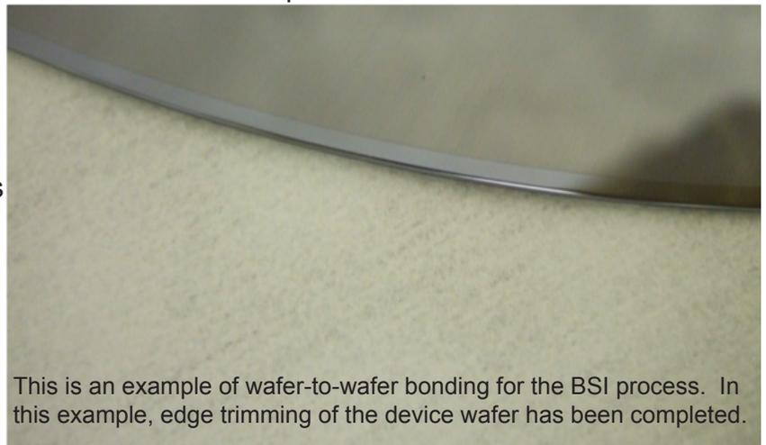
This is an example of wafer-to-wafer bonding for the BSI process. In this example, edge trimming of the device wafer has been completed.
