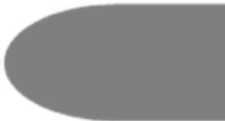
Classical "Bullet Nose" shape common to most semiconductor silicon wafer applications. (Drawing not to scale).
