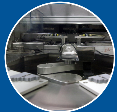
In-feed grinding w/wafer rotation
