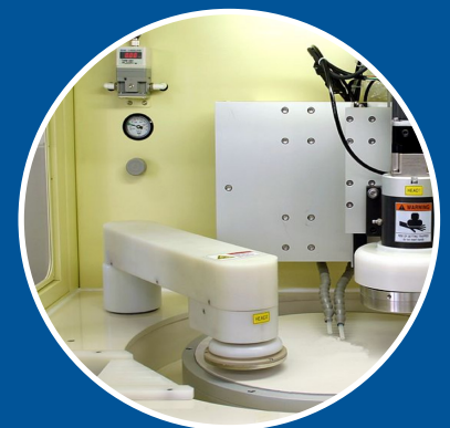
The POLI-500 Swing Arm Conditioning System for optimized CMP processing
